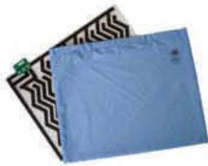
The Flexi-Pad Sensors have been specifically designed for laying in narrow voids (too small for point sensors) or wrapped around pipes at valves or joints where leaks are more likely to occur. The Flexi-Pad Sensor can be used singly, or in groups with a number of sensors being connected together to form one zone.
