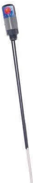
The Floodline Pipe-in-Pipe Sensor is based around a Point Sensor but designed for fitting into a female threaded socket provided at strategic points in the outer pipe. Short stainless steel probes extend into the cavity, or annulus, created between the inner and outer pipes. When liquid escapes into the cavity and contacts a sensor the alarm is activated. Two types of device are available for water and oil (oil/any liquid).
