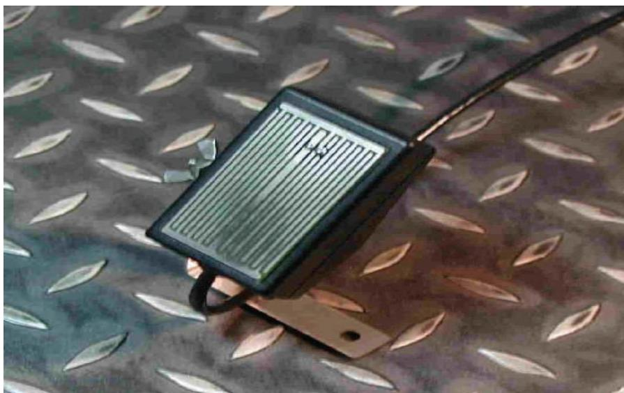
A totally weatherproof and self contained rain detection unit, which is used to signal when rain, hail or sleet is falling. Primarily used by the BMS industry to signal when skylights should be closed these units feature a heated detection comb to prevent the unit activating in frosty conditions or when dew is forming.
