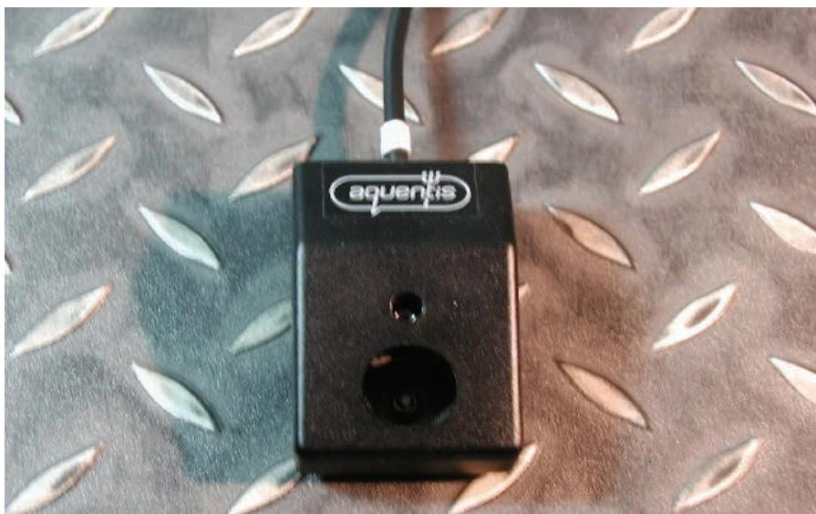
A totally self contained condensation detector designed to warn of the onset of condensation on a Chilled Beam air-conditioning system and thus preventing indoor rain damaging equipment and furnishings. One detector is needed for each point where cold water enters a ceiling so a large building may have several hundred condensation detectors.
