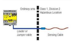
If protected by an agency approved zener barrier, TraceTek sensors in Class I, Division 1, Groups A, B, C, D Hazardous Locations (Zones 0 and 1 in Europe). Contact Tyco Thermal Controls to select proper zener barrier.
